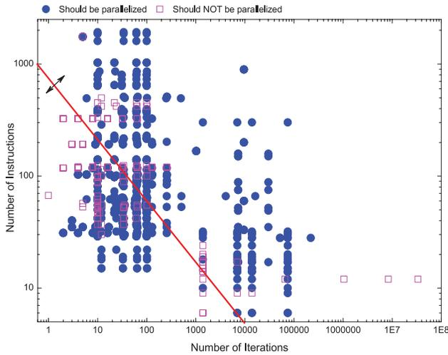
Fig. 5. This diagram shows the optimal classification (sequential/parallel execution) of all parallel candidates considered in our experiments for the Intel Xeon machine. Linear models and static features such as the iteration count and size of the loop body in terms of IR statements are not suitable for separating profitably parallelizable loops from those that are not.
