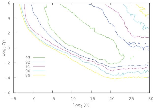
Fig. 7. Finding suitable SVM model parameters using grid search. In this contour map, each curve connects points of a pair of the two parameters that gives a particular prediction accuracy. The parameter setting that leads to the best prediction accuracy is chosen as the final model parameter.
